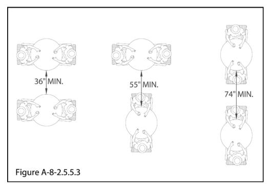
Figure A-8-2.5.5.3 illustrates the provisions of 8-2.5.5.3 of the Life Safety Code. This provides guidance on how aisles with movable chairs are to be measured, an issue that has often been questioned by enforcement officials.
